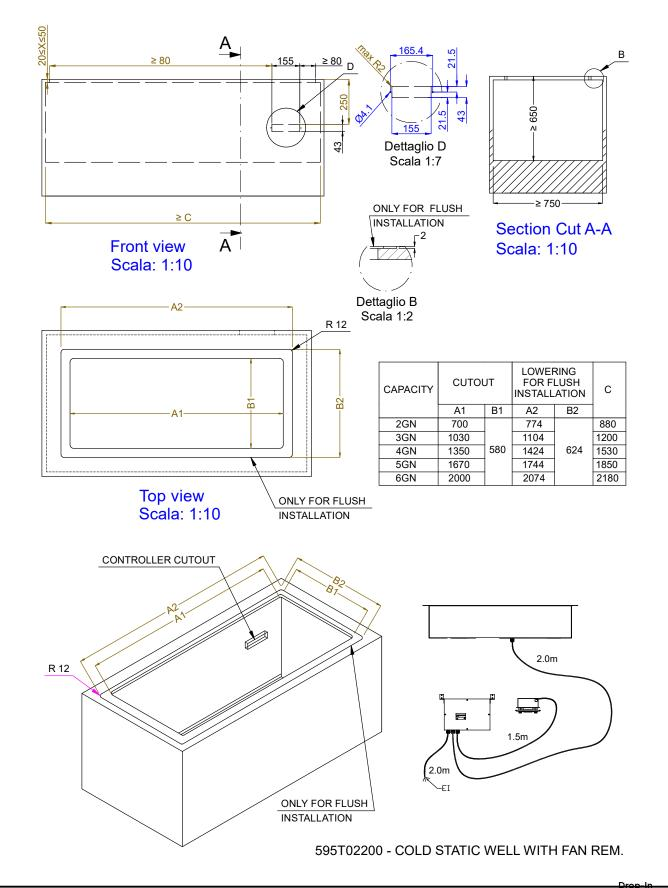
Drop-in remote refrigerated well, static with fan (5 GN container capacity) The company reserves the right to make modifications to the products without prior notice. All information correct at time of printing.
