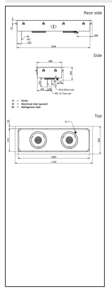
Drop-In Drop-in remote refrigerated well, static with fan (5 GN container capacity) The company reserves the right to make modifications to the products without prior notice. All information correct at time of printing.
